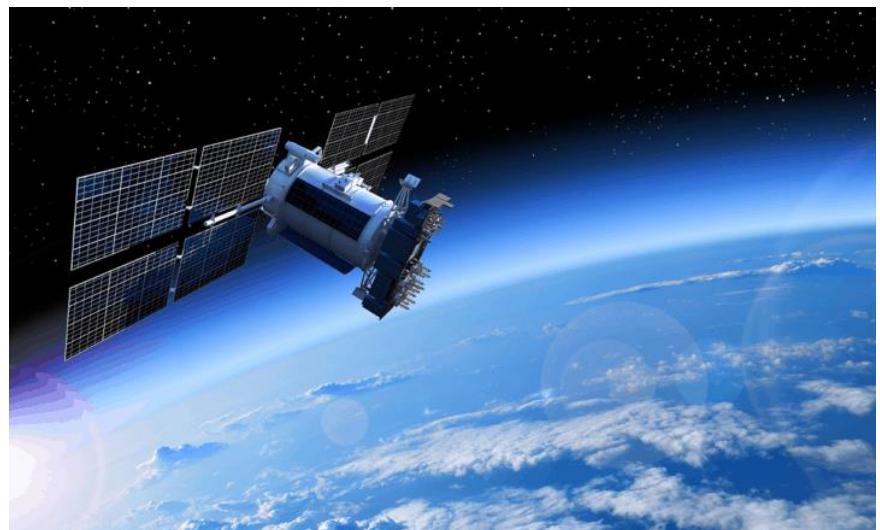
To calculate your 2-D position (latitude and longitude) and track movement, a GPS receiver must be locked on to the signal of at least 3 satellites. With 4 or more satellites in view, the receiver can determine your 3-D position (latitude, longitude and altitude). Once the user's position has been determined, the GPS unit can calculate other information, such as speed, bearing, track, trip distance, distance to destination, sunrise and sunset time and more.
